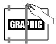
Remove remaining tape, remove remaining liner and squeegee using the same method in previous step.
